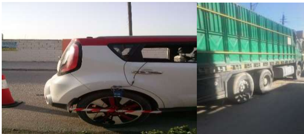
Figure 2. OBSI fixtures on Kia Soul and Mercedes Benz truck test vehicle.
